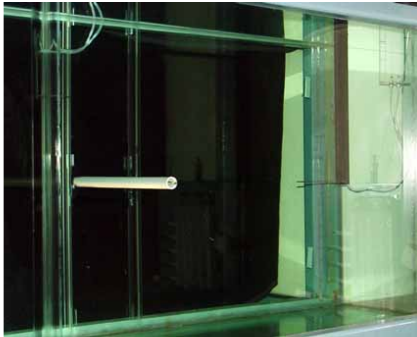
Figure 8: Photograph showing the circular cylinder model mounted in the RHRC 2436 water tunnel.
